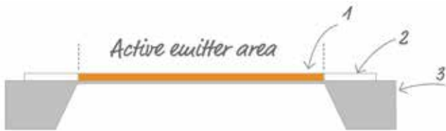
1 – Multi layer hot plate membrane containing NAC layer 2 – Bond pads 3 – Si frame and membrane
