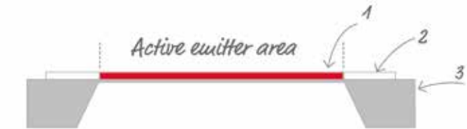
1 – Multi layer hot plate membrane containing CMOSI layer 2 – Bond pads 3 – Si frame and membrane
